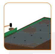
Install a suitable edging around all open sides. This could be a tanalised wooden edging, block paviours, granite setts, concrete path edgings or our very own flexible steel edging - CORE EDGE.
