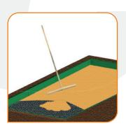
Cover the entire area with a 5-10mm bedding layer of sharp sand and compact. This layer will help to eliminate any minor undulations you may have in the subbase, it also helps to protect the underside of the grid from the subbase material.
