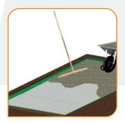
Fill the grid with your chosen aggregate either using a wheelbarrow or direct from a truck. Ensure the truck does not drive onto the grid. CORE PATH PRO is designed to be covered by a 10-15mm dressing layer of aggregate, making the grid virtually invisible. We recommend any angular aggregate up to 14mm in size.
