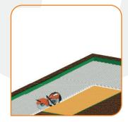
Install the CORE PATH panels, starting from one corner and working your way out, with the membrane facing down. Cut to shape using a petrol disc cutter or grinder. Please ensure to wear necessary PPE for the equipment being used.
