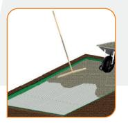
Fill the grid with your chosen aggregate either using a wheelbarrow or direct from a truck. Ensure the truck does not drive onto the grid. CORE PATH PRO is designed to be covered by a 10-15mm dressing layer of aggregate, making the grid virtually invisible.
