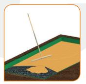
Cover the entire area with a 5-10mm bedding layer of sharp sand and compact. This layer will help to eliminate any minor undulations you may have in the subbase, it also helps to protect the underside of the grid from the subbase material.
