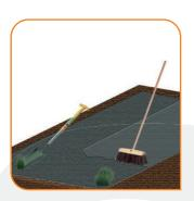
To install CORE PATH PRO over an existing old gravel, tarmacadam or concrete surface - you first need to clear the area of weeds and any loose material.
