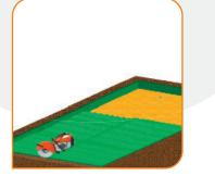
Install the grid starting from one corner and working your way out with the membrane facing down. Cut to shape using a petrol disc cutter or grinder. Please ensure to wear necessary PPE for the equipment being used.
