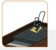
Install membrane and geogrid if required and then the subbase material. Ensure the subbase is well compacted using either a pedestrian roller or vibrating road plate.
