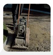
Repair the surface if there are any dips or pot holes with a suitable subbase material and recompact the entire area with a roller or vibrating road plate. If installing over tarmac or concrete, you may want to drill drainage holes in the surface to allow water infiltration.
