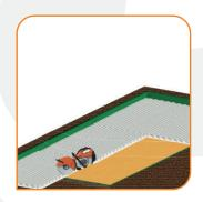
Install the CORE PATH panels, starting from one corner and working your way out, with the membrane facing down. Cut to shape using a petrol disc cutter or grinder. Please ensure to wear necessary PPE for the equipment being used.
