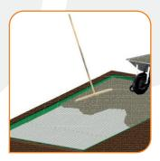
Fill the grid with your chosen aggregate either using a wheelbarrow or direct from a truck. Ensure the truck does not drive onto the grid. CORE PATH PRO is designed to be covered by a 10-15mm dressing layer of aggregate, making the grid virtually invisible.
