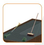
To install CORE PATH PRO over an existing old gravel, tarmacadam or concrete surface -you first need to clear the area of weeds and any loose material.
