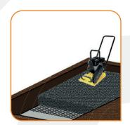
Install membrane and geogrid if required and then the subbase material. Ensure subbase is well compacted using either a pedestrian roller or vibrating road plate.
