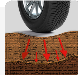
Downward pressure causes over compacted soil
