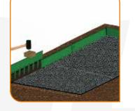
Install a suitable edging around all open sides. This can be tanalised wooden edging, block paviours, granite setts, concrete path edgings or our very own flexible metal edging - CORE EDGE.
