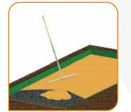
Cover the entire area with a 5-10mm bedding layer of sharp sand and compact. This layer will help to eliminate any minor undulations you may have in the subbase, it also helps to protect the underside of the grid from the subbase material.
