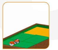
Install the grid starting from one corner and working your way out with the membrane facing down. Cut to shape using a petrol disc cutter or grinder. Please ensure to wear necessary PPE for the equipment being used.
