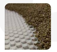
Install the grid starting from one corner and working your way out with the membrane facing down. Cut to shape using a petrol disc cutter or grinder. Please ensure to wear necessary PPE for the equipment being used. Fill the grid with your chosen aggregate either using a wheelbarrow or direct from a truck.
