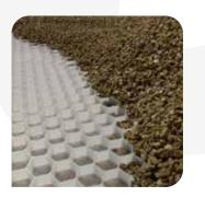
Fill the grid with your chosen aggregate using either a wheel barrow or direct from a truck. Ensure the truck does not drive onto the unfilled grid. CORE DRIVE is designed to be covered by a 10-15mm dressing layer of aggregate - making the grid virtually invisible.
