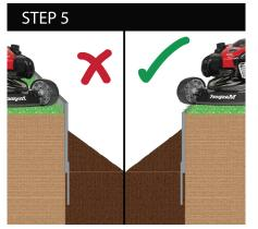
If using the edging on a lawn area the top of the edging should be flush with the soil to prevent the lawn mower blade making contact with the top of the edging. STEP 3
