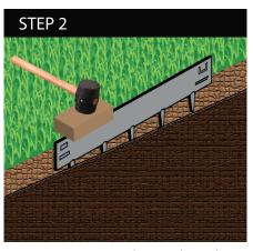
Starting at one end, tap the edging down using a wooden block and mallet. Ensure the edging remains vertical as it is driven into the ground, this prevents twisting when it comes to installing your next edging.
