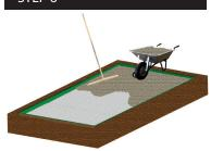
Fill the grid with your chosen aggregate either using a wheelbarrow or direct from a truck. Ensure the truck does not drive on unfilled cells. CORE Drive is designed to be covered by a 10-15mm dressing layer of aggregate making the grid virtually invisible
