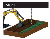
Excavate area for subbase to be installed. For subbase calculation see overleaf. Ensure to allow for: 10mm sand bedding layer; depth of grid and the 10-15mm dressing of aggregate when calculating depth from surrounding surfaces.
